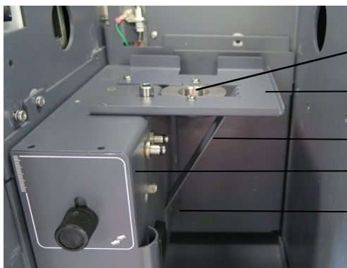
Figure 20. Workhead bracket fitted to the burner adjuster
