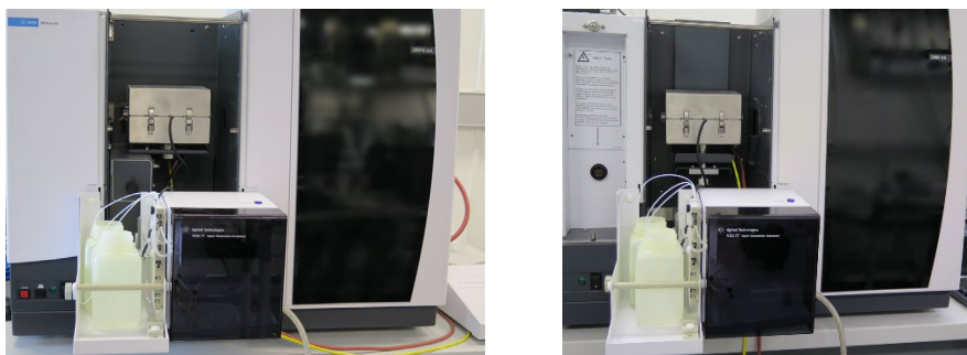
Figure 1. Installed ETC with VGA on a Flame (left) and Zeeman (right) instrument
