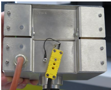
Figure 24. Temperature cable connected to the workhead. An older style cell heater cable is shown.
