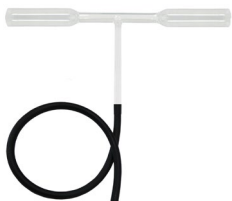
Figure 28. Black fluoroelastomer tubing on the inlet cell stem
